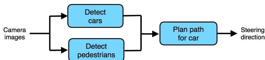
It has three components: One detects other cars using the camera images; one detects pedestrians; then a final component plans a path for our own car that avoids the cars and pedestrians.
